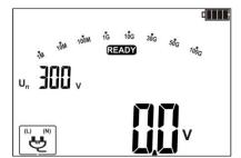
After inserting WS-04 into the socket, the screen displays a message indicating the detection of the adapter.
