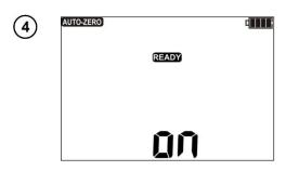
are displayed, confirming the completion of test leads resistance compensation.
