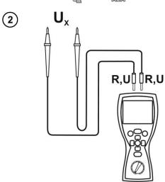
Connect the meter to a voltage source.
